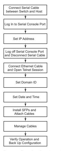
Figure 17. Flow of configuration tasks for the SAN384B
